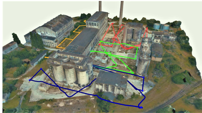
Fig. 1: 3D-view of the proposed system guiding safe and successful navigation of a team of four UAV-agents (with trajectories shown in different colors) in a photo-realistic simulation of an industrial site, despite that the user-defined waypoints for the UAVs correspond to partially overlapping regions. Via hierarchical planning, the proposed system is able to safely plan the UAVs' paths, running state estimation and local obstacle avoidance onboard each UAV, and sensor fusion and multi-robot global planning on the server to collect all UAVs' experiences in a joint, optimized map.
