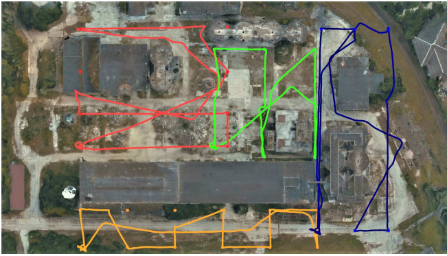
Fig. 4: Top view of the simulation with four agents. Four different regions were selected and each arbitrarily assigned to one of the agents. As the waypoints were chosen to form a lawnmower pattern, some of them lie inside obstacles (e.g. buildings). The global planner successfully identified and skipped these positions while reaching the accessible remaining points of interest.
